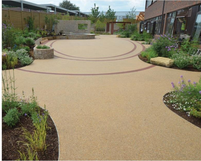
Primary Paving - Resin Bound Gravel
