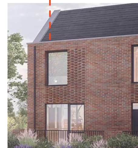
Protruding brick header bond detail to selected areas on front elevations
